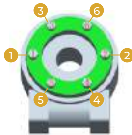
FIGURE 4. BOLT TORQUE SEQUENCE
